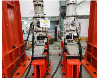
Figure 1: Concrete Sleeper Test Set Up
