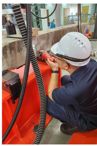
Figure 3: Competent technician examines the concrete sleeper sample for cracks during the test.
